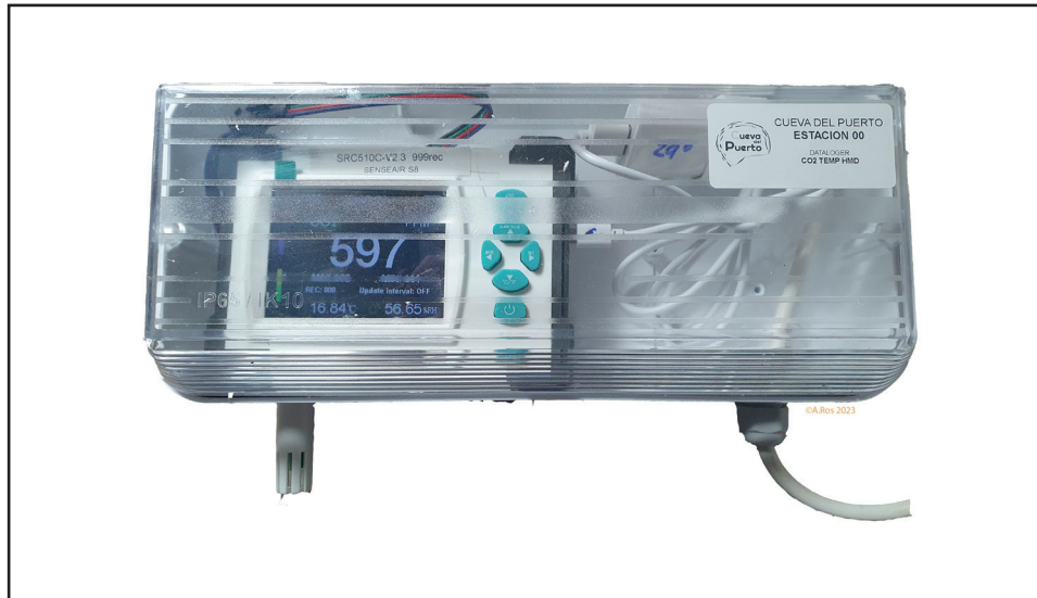
Photo 2: Carbon Dioxide Detector measuring station adapted to Zemper IP66 waterproof box.
