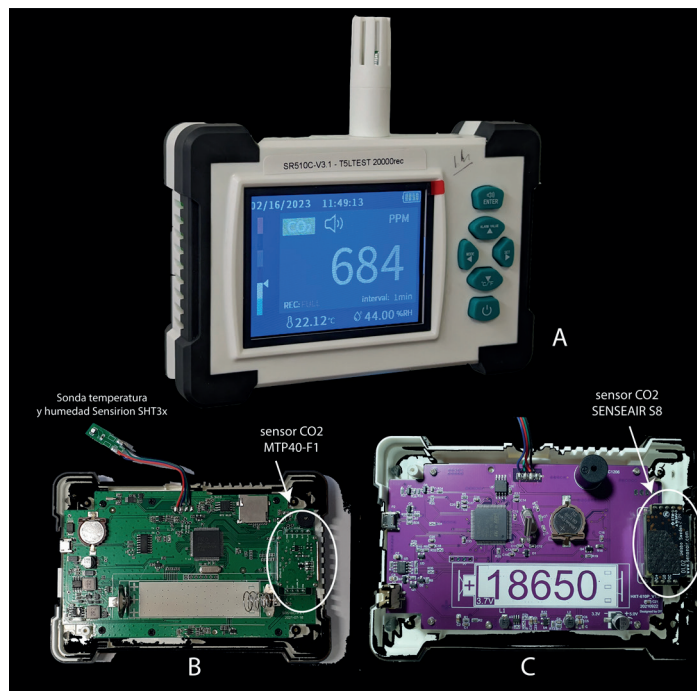
Photo 1. A CO 2 , temperature, and humidity datalogger (EcoDeyi) with two CO 2 sensors models: MTP40-F1 and SENSEAIR S8.
