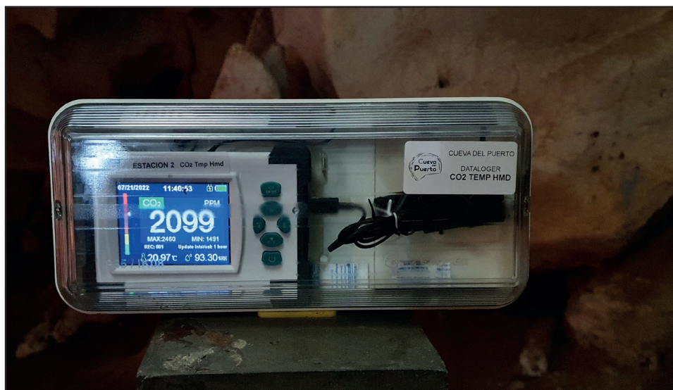
Photo 5. Carbon Dioxide Detector equipment installed inside Cueva del Puerto (seven-month operating period).
